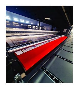
Large-calibre rolls and a take-up system designed to handle heavy materials with ease, enabling seamless roll material printing. A smart media guide ensures precision for flatbed materials.
